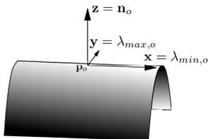
Fig. 4. The right-handed orthogonal coordinate system constructed from the surface normal  $\mathbf{n}_o$  at the mesh point  $\mathbf{p}_o$  and the local range directions  $\lambda_{min,o}$  and  $\lambda_{max,o}$ .
