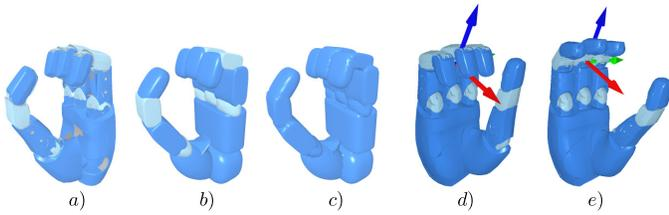
Fig. 2. Original model of the hand (a), remodeled with superellipsoids (b), and the final manifold mesh (c). The distance between two adjacent points of the grid was set to  $2.2mm$ . The first (d) and second (e) hand preshapes that were used for grasp computation in section VI. The frames of the hand surface patches — inputs to the surface matching algorithm — are also shown, where the red arrows represent the surface normals at the patch centers.
