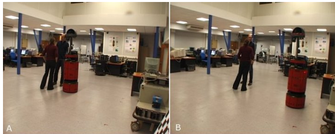
Fig. 9. A comparison between a classic motion planner and the human-aware navigation planner. Clearly the last one produces more acceptable path by taking into account the safety and visibility of each human in the environment
