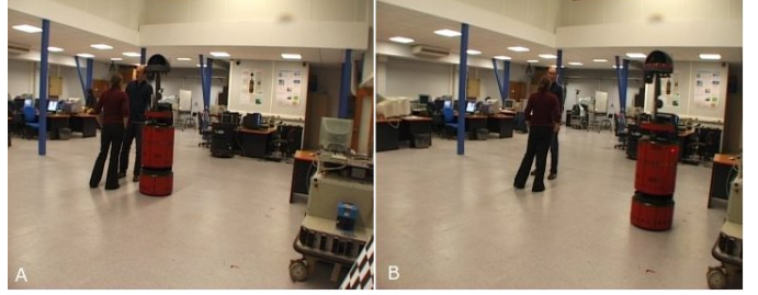
Fig. 9. A comparison between a classic motion planner and the human-aware navigation planner. Clearly the last one produces more acceptable path by taking into account the safety and visibility of each human in the environment
