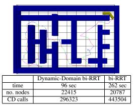
Fig. 10. The goal in this example is to move a two link articulated body with 4 degrees of freedom from one corner of the labyrinth to another.
