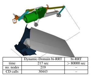
Fig. 9. An example from the manufacturing industry. The goal is to find a collision free path dismounting a wiper motor from a car body.
