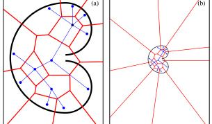
Fig. 1. Trees constructed by an RRT-based planner and the Voronoi regions associated with the nodes of the trees. (a) A bug trap problem in high dimensions can be a challenging problem for this planner. (b) It becomes much more challenging when the region for sampling is enlarged.
