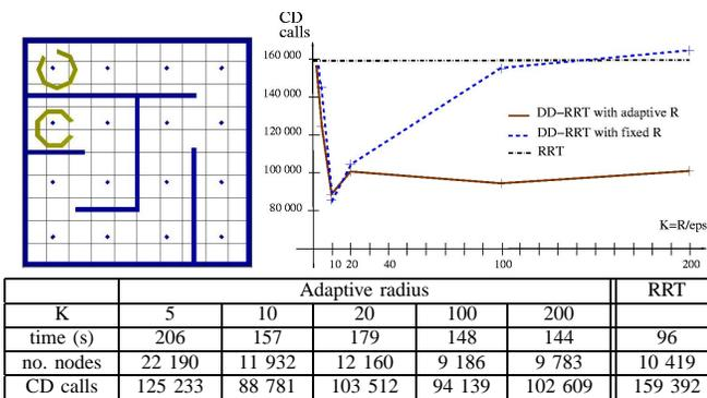
Fig. 9. Results for a maze environment. The C-shaped robot has to move from one extremity of the maze to the other by combining rotations and translations.
