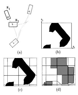
Fig. 9. (a) Two  $\mathcal{S}\mathcal{A}$  paths. (b) The coordination diagram. (c) The partition of the diagram induced by the path decomposition. (d) The bounding box representation of the obstacles and a solution path.
