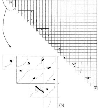
Fig. 15. A case with 32 robots: (a) the robots traces and (b) the 496 elementary diagrams. The partition into the eight robot subgroups is illustrated by the eight bold triangles.
