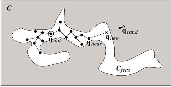
Fig. 2. Illustration of one expansion step of a search tree using an RRT-based algorithm. The tree tends to cover  $C_{feas}$ : the feasible subset of the search-space  $C$ .
