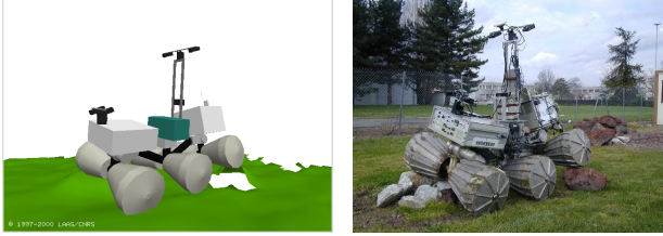
Figure 9: A predicted placement of the robot on the DEM (left), and the corresponding placement in reality (right).
