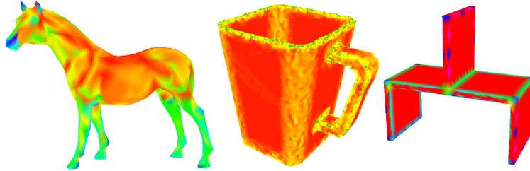
Figure 8: The mean curvature of the object surface is used as a quality criterion on the contact position. Surface color varies from red (low curvature, good location) to blue (high curvature, bad location), through green.
