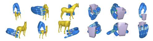
Figure 9: Some of the various grasps that were computed for objects with complex shape. Friction cones are also represented.
