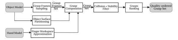
Figure 1: Overview of the proposed method to compute a set of grasps from object's and hand's models.
