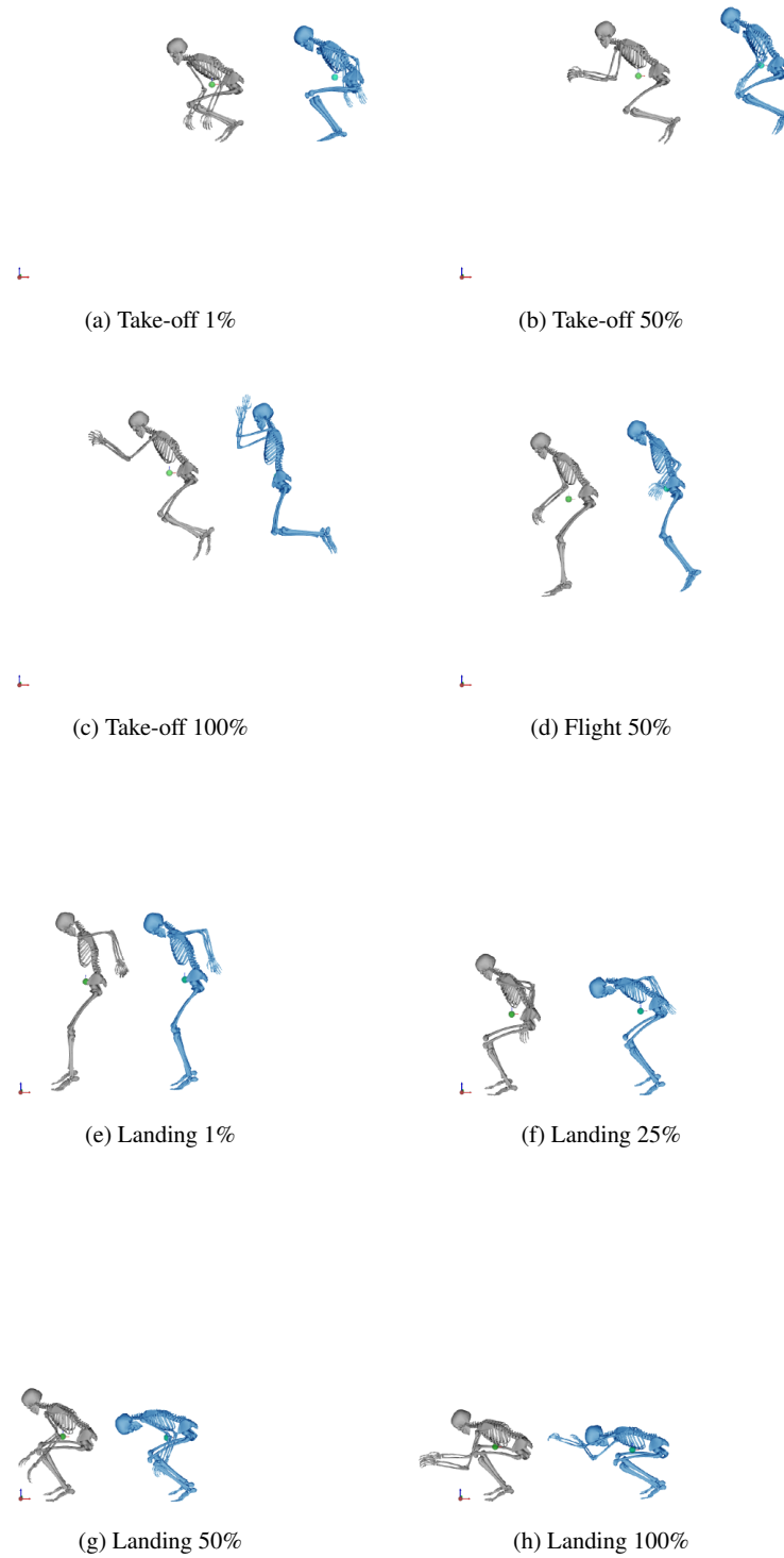
Fig. 3: Snapshots of the take-off phase (a)(b)(c), flight phase (d), and landing phase (e)(f)(g)(h) at different percentages of the motion phases. The skeleton on the left, represents the result of the inverse kinematics from motion analysis of a Parkour practitioner, whereas the skeleton on the right is the motion generated through hierarchical control.
