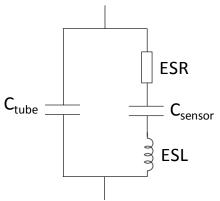
Fig. 7. Electrical model of the sensor
