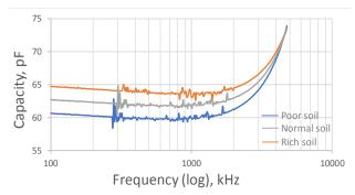
Fig. 5. Capacity according to the salinity
