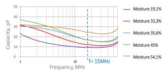
Fig. 6. Capacity according to moisture
