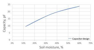
Fig. 3: Capacity response of the capacitor design
