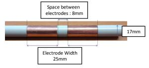
Fig. 2. Optimized capacitor design
