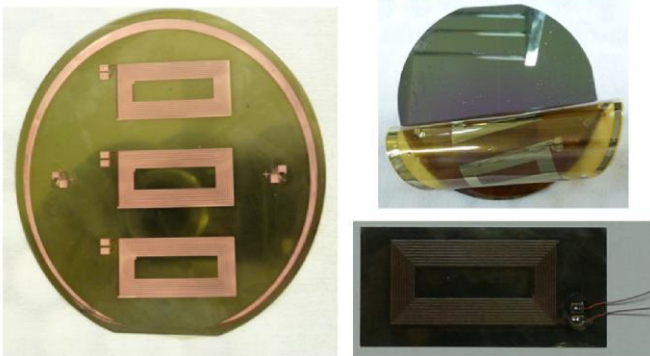
Fig. 7. Silicon wafer with three flex printed coils.
