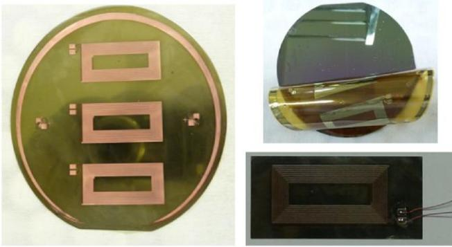
Fig. 7. Silicon wafer with three flex printed coils.
