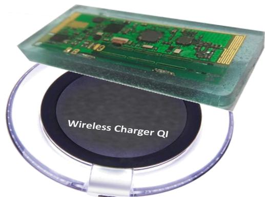
Fig. 6. Wireless charging of the encapsulated electronic patch
