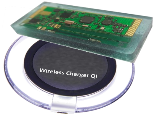
Fig. 6. Wireless charging of the encapsulated electronic patch
