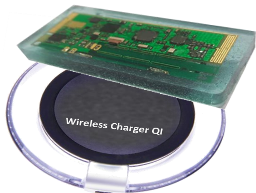
Fig. 6. Wireless charging of the encapsulated electronic patch
