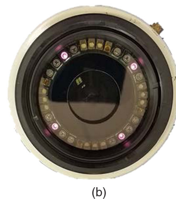
Fig. 2 LEDs included in the ring of the multispectral system: (a) spectral emission and (b) front picture of the ring.
