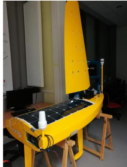
Fig. 1. IBOAT3 is a fully autonomous sailing boat. Length: 1.8 m, height: 2 m, weight, 35 kg. Electrical power is provided by a 0.65 m<sup>2</sup> solar panel
