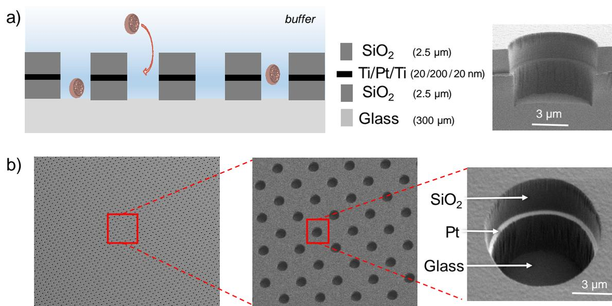
**Figure 1**– (a) left: Scheme of the OptoElecWell array for the monitoring of single mitochondria activities, right: Cross-sectional SEM view of a typical microwell; (b) SEM images of the  $\text{SiO}_2$ -based microwell array (mean diameter:  $6\ \mu\text{m}$ ; mean depth:  $5.2\ \mu\text{m}$ ) with integrated platinum-ring nanoelectrodes (thickness:  $\sim 200\ \text{nm}$ ) on a glass substrate.
