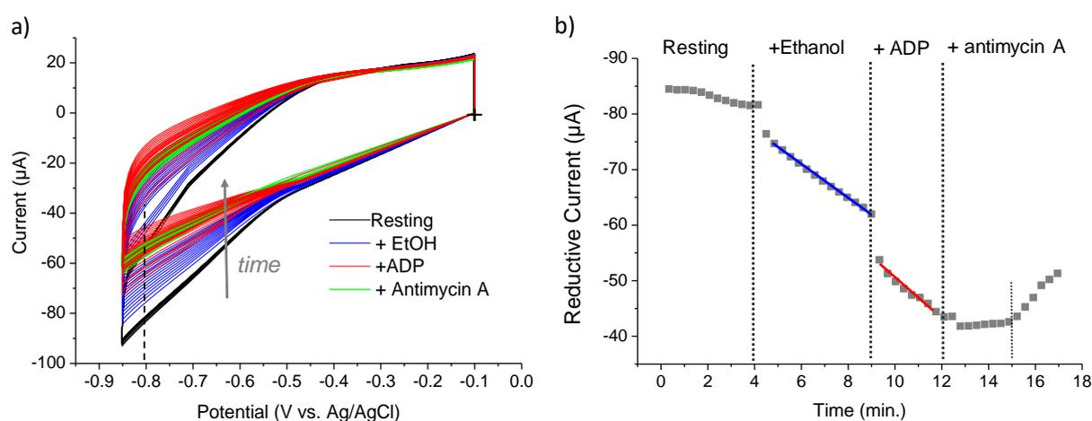
**Figure 5-** (a) Electrochemical monitoring of the oxygen consumption by mitochondria present in the OptoElecWell device under different stages (Scan rate: 4 V.s<sup>-1</sup>, delay of 10 sec. between scans). (b) Evolution of the reduction current at -0.8 V vs Ag/AgCl measured on each scan, following additions of bioenergetic substrates (Ethanol, ADP) and an inhibitor (antimycin A). Measurements were conducted simultaneously to NADH ones reported in Figure 4.
