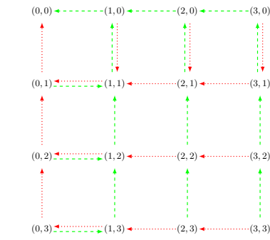
Figure 3: Two arc-disjoint arborescences as in Lemma 1 for a finite 4 \times 4 grid, with destination t = (0, 0) and roots r_1 = (1, 0) , r_2 = (0, 1) . The arcs of the trees T_1 and T_2 are drawn in green (dashed) and red (dotted), respectively.
