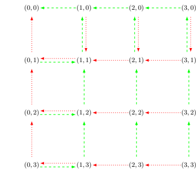
Figure 3: Two arc-disjoint arborescences as in Lemma 1 for a finite 4 \times 4 grid, with destination t = (0, 0) and roots r_1 = (1, 0) , r_2 = (0, 1) . The arcs of the trees T_1 and T_2 are drawn in green (dashed) and red (dotted), respectively.
