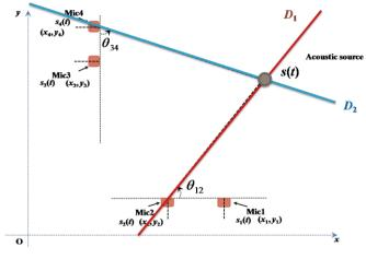
Fig. 3. Two 2-microphone pairs array
