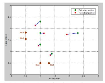
Fig. 9. Acoustic source estimated positions vs theoretical positions
