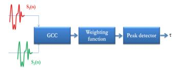
Fig. 10. Estimation of TDoA using the GCC method
