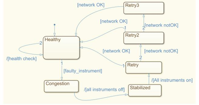
Fig. 8: Original statechart for the Spacewire Network FDIR
