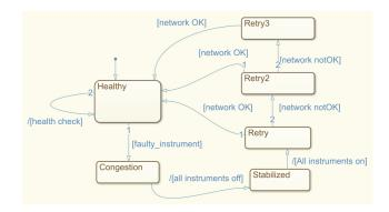
Fig. 8: Original statechart for the Spacewire Network FDIR
