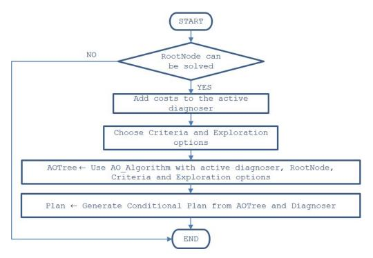
Fig. 5: AO main Algorithm flowchart
