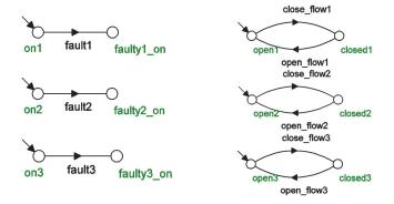
Fig. 7: Supremica automata for instruments and SpaceWire router
