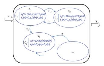
Fig. 3. Example of a hybrid system.
