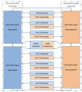
Fig. 2. Spacewire Network architecture
