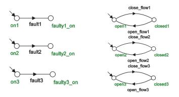
Fig. 7: Supremica automata for instruments and SpaceWire router
