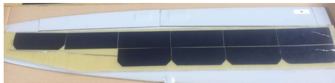
Fig. 12 Final encapsulation of PV cells
