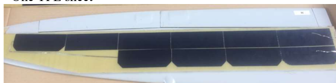
Fig. 12 Final encapsulation of PV cells
