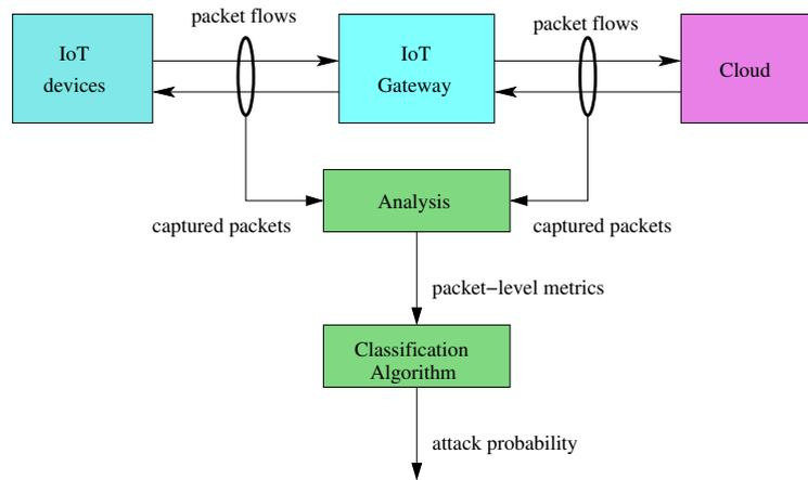
Fig. 1: Architecture of the online attack detection system..
