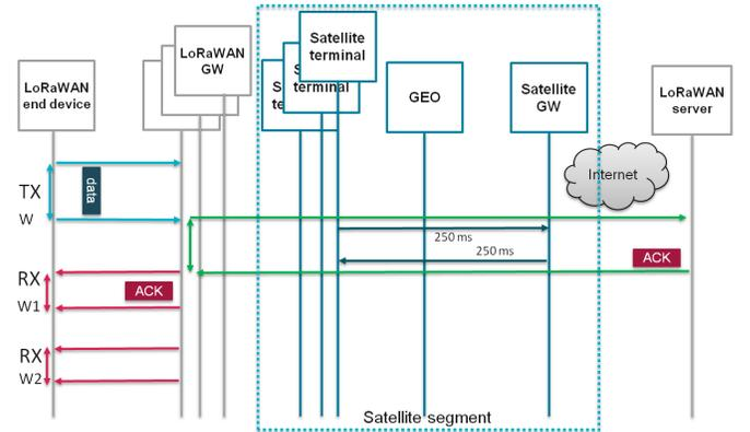
Fig. 4. LoRaWAN Mode A with satellite backhaul
