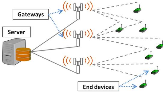
Fig. 1. LoRaWAN architecture
