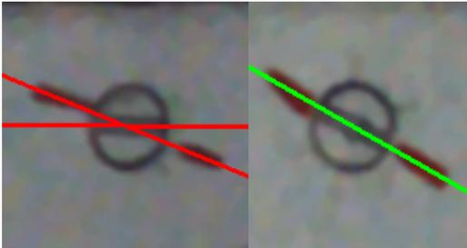
Figure 8: Detection of a loose and tight screw.
