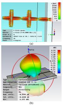
Fig. 2. (a) Electric field distribution and (b) 3D radiation characteristic at 94 GHz
