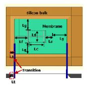
Fig. 1. Layout of the membrane suported double folded slot antenna
