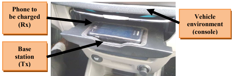
Fig. 2. Illustration of a WPTS in a vehicle environment
