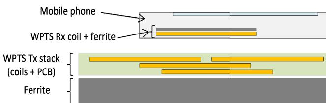
Fig. 3. Schematic of Tx coils assembly coupled with the Rx system
