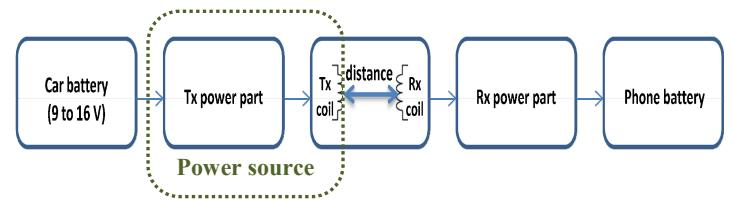
Fig. 1. Schema of a typical inductive WPTS
