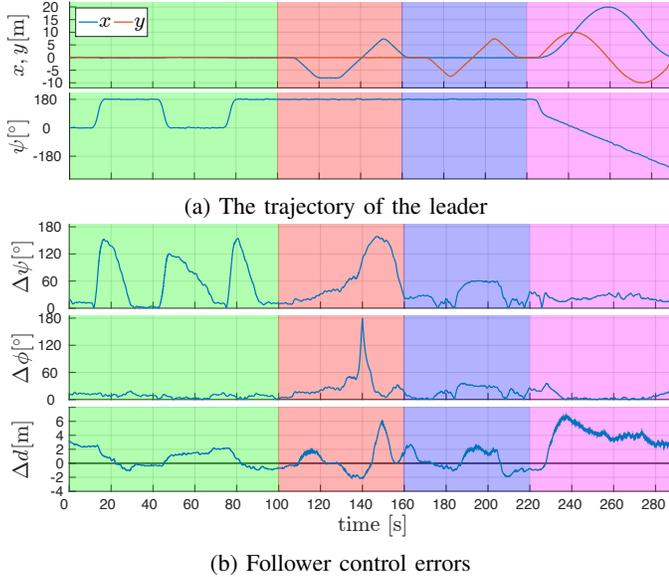
Fig. 10: (a) The leader trajectory defined by position and yaw  $\psi$ . The height was constant, set to 8 m. (b) From top to bottom - tailing error, heading error and distance error. Colored zones correspond to specific leader motions - rapid rotation (green), retreat-approach (red), left-right (blue), and circle following (purple).
