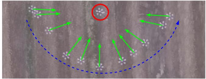
Fig. 1: Top view of a *directed leader-follower* experiment. The leader rotates by  $180^\circ$ . This is detected by UVDAR sensor carried by the follower, triggering it to create a trajectory as per the proposed algorithm in order to preserve its pose in the leader frame.
