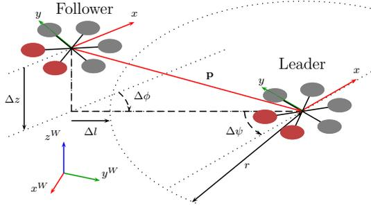
Fig. 5: Variables defining our requirements on the leader-follower system. Red propellers denote the back of the UAV. We want the leader to be on the circular perimeter with the radius  $r$  around the leader ( $\Delta l \rightarrow 0$ ) at the height of the leader ( $\Delta z \rightarrow 0$ ), while facing it ( $\Delta \phi \rightarrow 0$ ) from its back ( $\Delta \psi \rightarrow 0$ ).
