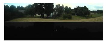
Fig. 2: Comparison between visible and UV camera footage from UVDAR, collected during the experiment. The UV image is significantly easier to process to retrieve UAV information.
