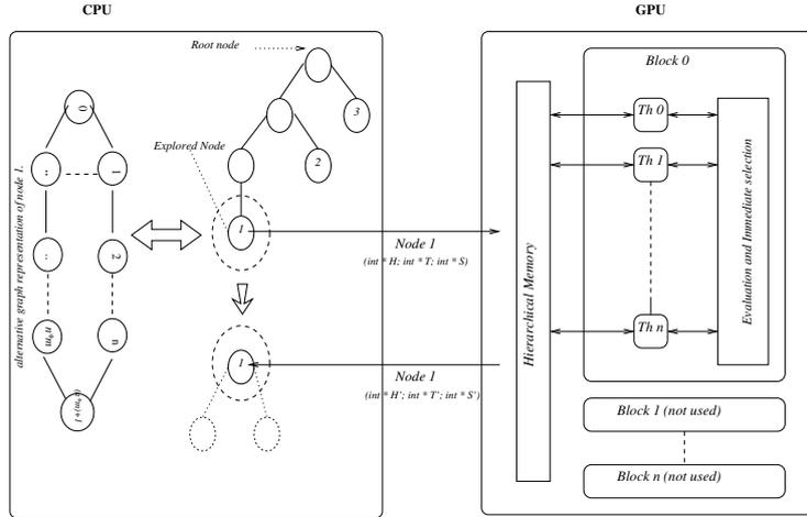
Figure 9: GPU Evaluation of a single node.
