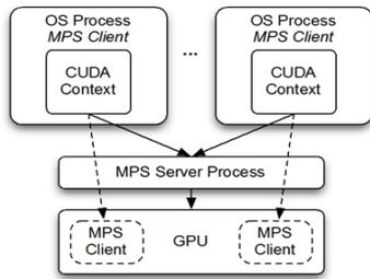
Figure 12: MPS components.
