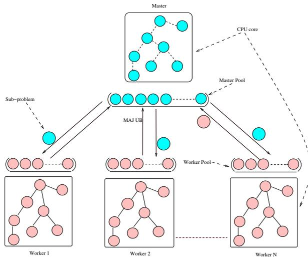
Figure 8: Global architecture of the proposed Master/Worker parallelization.
