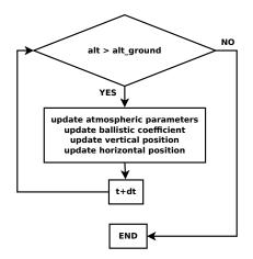
Figure 5. Envelope drift descent calculation
