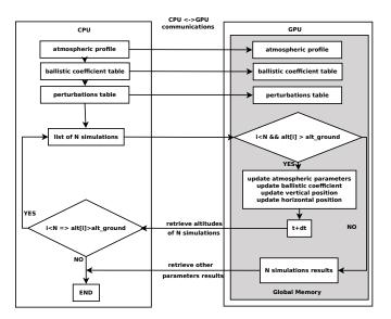
Figure 6. GPU loop parallel algorithm
