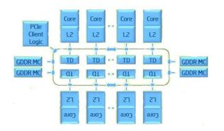
Figure 2. Microarchitecture of the MIC coprocessor
