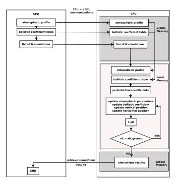
Figure 7. GPU task parallel and memory management algorithm
