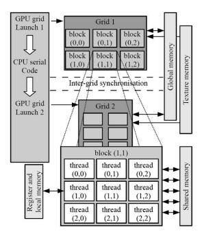
Figure 1. Thread and memory hierarchy in GPUs
