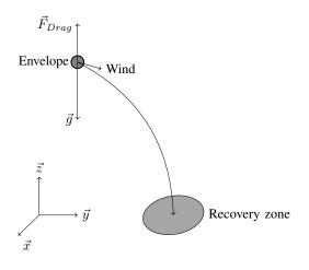
Figure 4. Sketch of drift descent motion dynamics
