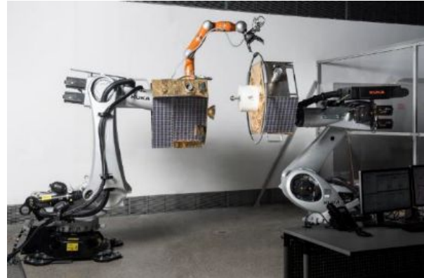
Figure 6. Ground test facility of DLR for visual target tracking when approaching a target in close-range approach and visual servoing
