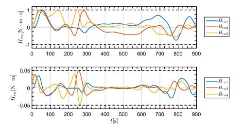
Figure 11: Reaction wheels angular momentum and its variation of scenario 2 for the first random realization
