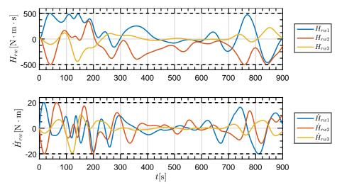
Figure 7: Reaction wheels angular momentum and its variation of scenario 1 for the first random realization
