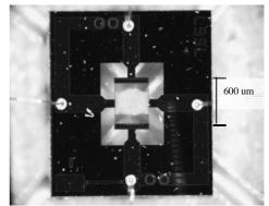
Fig. 1. Top view of the complete SnO, gas sensor
