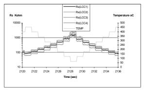
Fig. 6. Triangular temperature profile and sensors response
