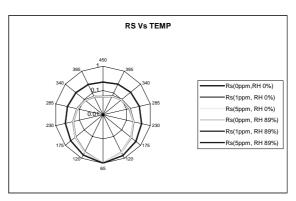
Fig. 7. Normalised temperature response at 0 and 90% of RH
