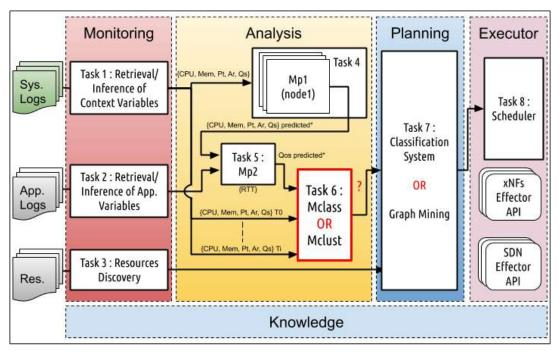
Fig. 2: General Controller - Autonomic Cycle for QoS provisioning.
