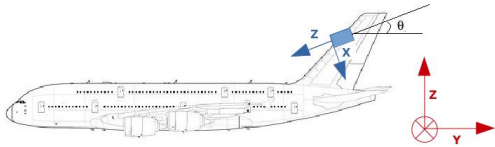
Figure 2: Representation of the camera coordinate system (blue) and IPM coordinate system (red)
