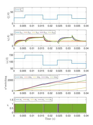
Fig. 6: From the top, the following evolutions: current reference of the leader  $\mathcal{N}_1$ ,  $i_{b,i}^r$ , output currents of each node,  $i_b$ , demanded current  $i_d$ , number of switching of each node and discrete input variables  $\sigma_i$ .
