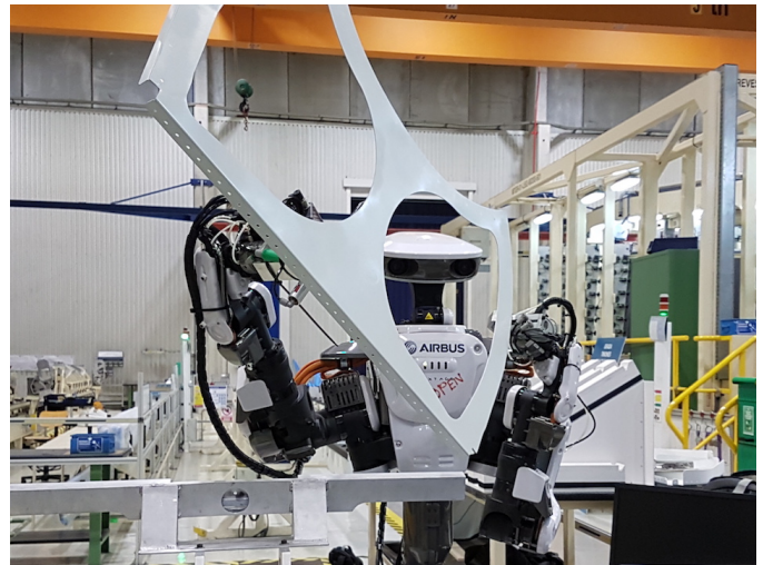
Fig. 1: The Nextage robot is manipulating a rib with both arms to place it on the deburring support.
