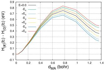
Fig. 5: Energetic path of diffusion of  $V_0^{-2}$  under different electric field orientation. Different colors address the enthalpy variation along the path when an electric field of 3.6 MV.cm<sup>-1</sup> is applied along different directions ( $\pm$  orthogonal axis of the box).
