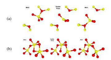
Fig. 3: (a) migration of charged +2 Oxygen Vacancy  $(V_O^{+2})$ , (b) migration of a charged -2 Oxygen Interestitial  $(I_O^{-2})$ .
