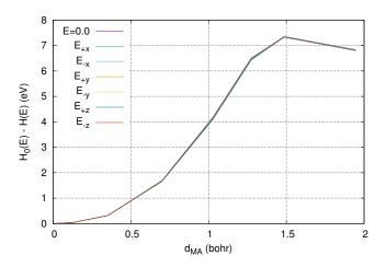
Fig. 2: Formation path of a neutral Frenkel pair (FP),  $V_OI_O$ , from a -Si-O-Si-O- quartz structure. Different colors address the enthalpy variation along the path when an electric field of 3.6 MV.cm<sup>-1</sup> is applied along different directions ( $\pm$  orthogonal axis of the box).
