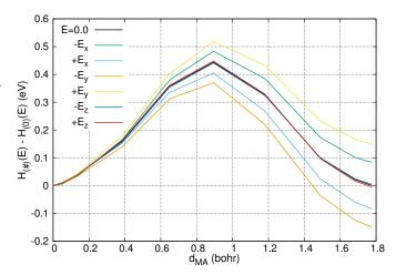
Fig. 4: Energetic path of diffusion of  $I_O^{-2}$  under different electric field orientation. Different colors address the enthalpy variation along the path when an electric field of 3.6 MV.cm<sup>-1</sup> is applied along different directions ( $\pm$  orthogonal axis of the box).
