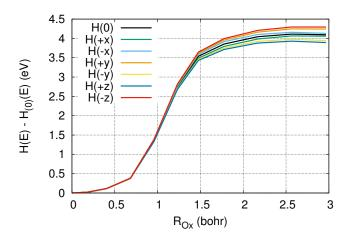
Fig. 1: Formation path of a charged Frenkel pair (CFP),  $V_O^{+2}I_O^{-2}$ , from a -Si-O-Si-O- quartz structure. Different colors address the enthalpy variation along the path when an electric field of 3.6 MV.cm<sup>-1</sup> is applied along different directions ( $\pm$  orthogonal axis of the box).
