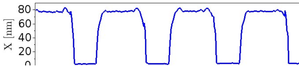
Fig. 4. Atomic-Force Microscope measurement of the profile of the etched grating into the SiN layer.
