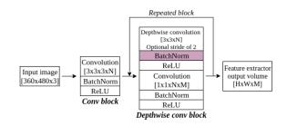
Figure 2: MobileNetv1 consists in stacking a convolutional block followed by multiple depthwise blocks. The purple "BatchNorm" block was removed in our modified version.
