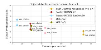
Figure 5: Frames per second on Titan Xp vs. Mean Average Precision. Detectors are tested with different feature extractors on both min\_clutter and max\_clutter test sets. We observe close performances between sets for each detector, and a correlation between precision and execution speed – Faster R-CNN + ResNet being the most precise but slowest detector and SSD the fastest but less precise one.
