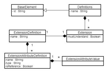
Figure 2. Extension class diagram (OMG, 2013)
