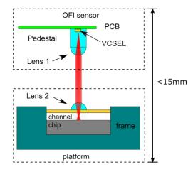
Figure 1. Schematic of the miniaturized optical feedback interferometry (OFI) flowmetry sensor system.
