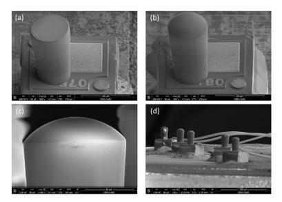
**Figure 3.** Scanning electron microscope images of VCSEL chip, including a micro-optical element. (a) after 80  $\mu$ m-diameter DF-pedestal fabrication, (b) after lens fabrication with self-centering on the pedestal surface, (c) zoom on microlens profile, (d) general view of lensed-devices after final bonding step.
