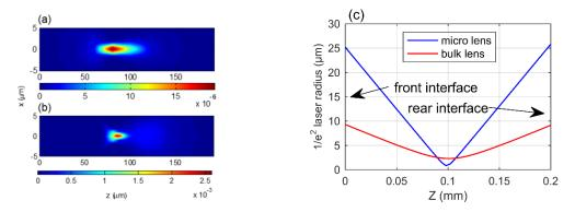
**Figure 6.** Modeling of laser incidence irradiation profile in the cross-section of the microchannel (X-Z plane) (ZEMAX). (a) Via bulk glass optical setup, (b) via miniaturized microlens set-up, (c) laser beam waist radius profile through the microchannel along the Z direction in both cases.
