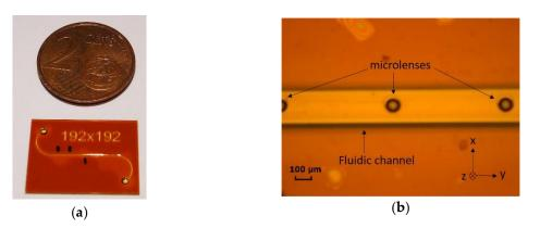
**Figure 5.** Photograph of the microfluidic chip: (**a**) View of the entire serpentine channel chip and size comparison with a coin of 0.7 inches in diameter (**b**) Zoom on the central part of the microchannel with focusing microlenses deposited on the surface. The lenses are positioned at the center of the channel in the X direction and spaced 500  $\mu$ m apart in the Y direction.
