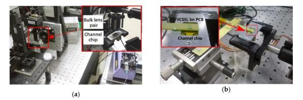
**Figure 7.** Comparative schematic of the OFI flowmetry sensor setups in microfluidic measurements. (a): Conventional commercial bulk lens-pair-based system. The inset presents the optical arrangement. (b): Integrated VCSEL-based system involving the sensor and a micromechanical stage for lateral position adjustment. The inset displays the fluidic platform and the backside of the PCB with lensed VCSEL.
