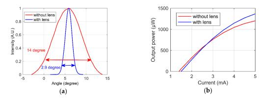
**Figure 4.** Characterizations of VCSELs without microlens (in blue), with microlens (in red). (**a**) Full  $1/e^2$  divergence angles at 3 mA current (**b**) Output current plotted as function of the current applied to the VCSEL.
