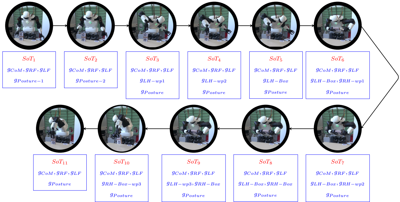
Fig. 6. Stack-of-Tasks sequence found by the Agimus system (simplified view)
