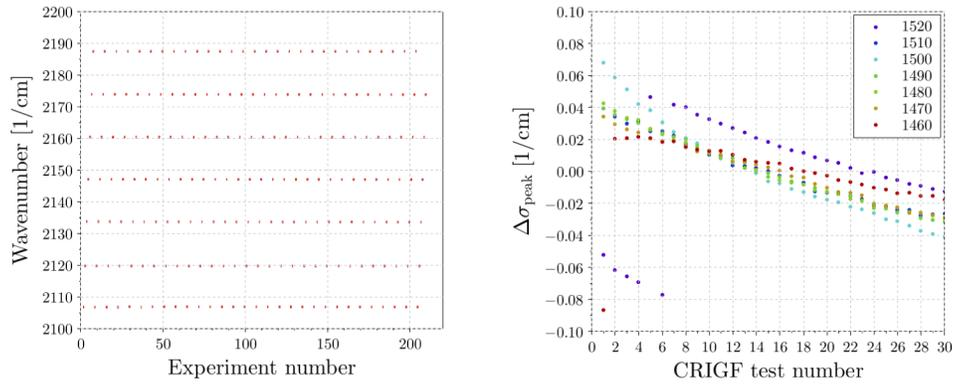
**Fig. 8.** Left : emitted spectrum as a function of the registered position while scanning 30 times over the 7 CRIGFs providing spectral stabilization. Right : change of peak wavenumber  $\sigma_{\text{peak}}$  during the scan presented in left figure. Each color corresponds to one CRIGF (GC period in the legend caption). The indicated change is relative to the average wavenumber over the scans for each CRIGF.
