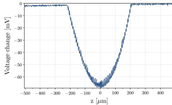
**Fig. 3.** Change in the voltage  $V$  between QCL contacts for a fixed injection current of  $I = 320$  mA as a function of the position of the sample along the optical axis.  $z = 0$  corresponds to the image plane where the bias voltage reaches a minimum.
