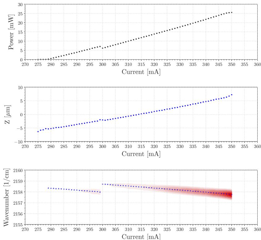
**Fig. 10.** Top : total emitted power versus injected current. Middle : variation of the  $Z$  position of the CRIGF for each current, with respect to its mean position. Bottom : emitted spectrum versus injected current in white to red linear color scale. The crosses correspond to the emission maximum.
