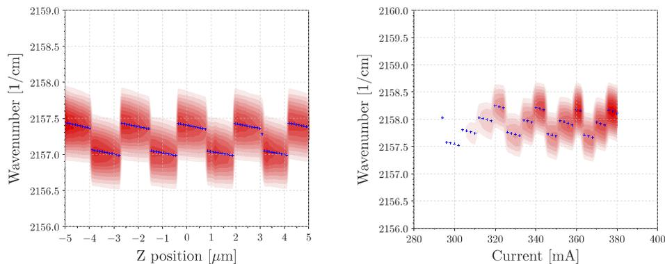
**Fig. 9.** Left : evolution of the spectra (color map, white to red, linear scale in arbitrary units) for increasing length of the cavity for the CRIGF with best overlap with the gain (1480 nm period). The injected current was 340 mA. The peak wavenumbers are reported as blue crosses for each acquired spectra. Right : evolution of the spectra with the injected current, for the same CRIGF, with the same conventions as left figure.
