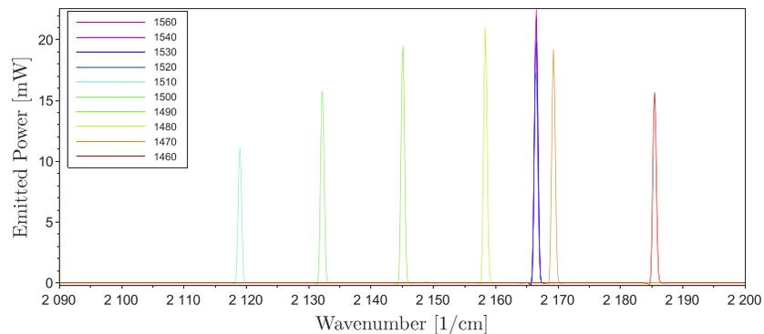
**Fig. 5.** Evolution of the emitted spectrum as a function of the GC period for a GC filling factor of 45 %. The vertical axis is normalized to the total emitted power.
