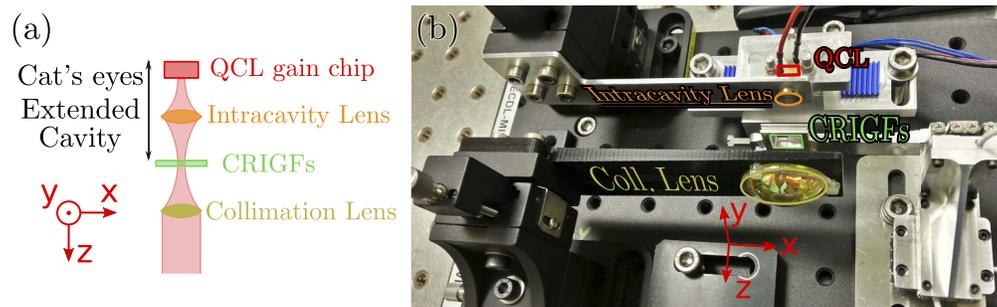
**Fig. 2.** (a) schematic of the cat's-eye quantum cascade extended cavity; (b) corresponding top view.
