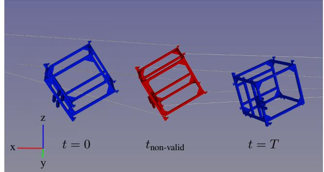
Fig. 1: Visualization of a path of the CDPR CoGiRo, parametrized by  $[0, T]$ . The first and last poses of the path are valid (blue). The continuous tension validation has found a non-valid pose (red) at parameter  $t_{\text{non-valid}}$ , therefore the path is not valid. Cables (grey) are shown only for the red pose.
